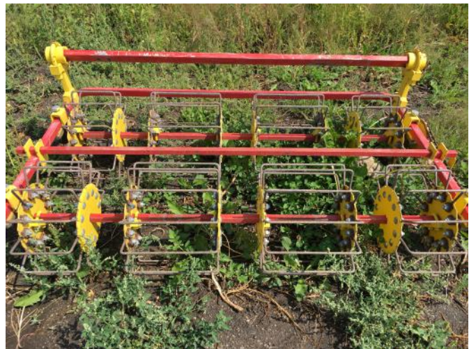
At Fourth Wave, the spacing on the Buddingh is set for three crops rows spaced 15" apart
