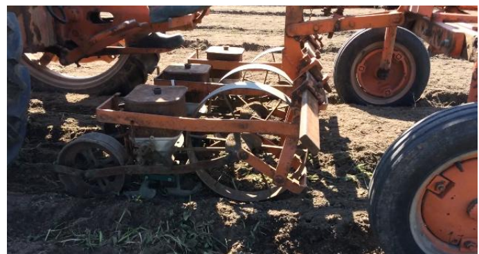
Planet Jr Seeder, belly-mounted on the Allis Chalmers
