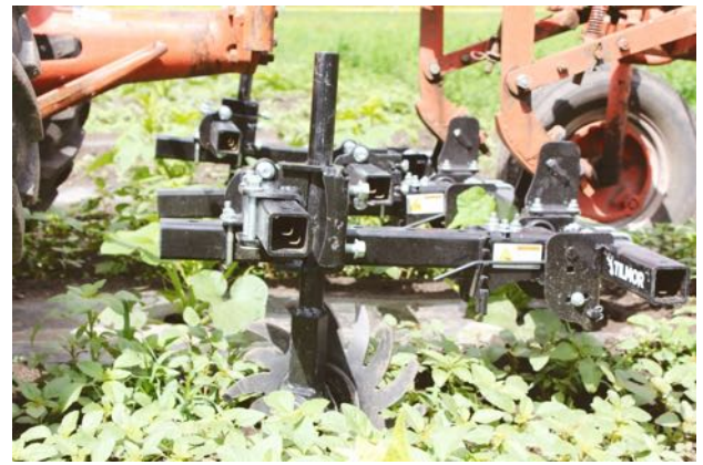
The spyder, belly-mounted to Randi's Allis Chalmers tractor. Note 1.5" tool bar and tool clamps.
